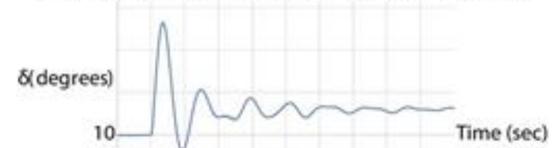
Generator Rotor Angle Swings Following Disturbance
