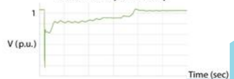
Substation Voltage Profile Showing Fault and Delayed Recovery
