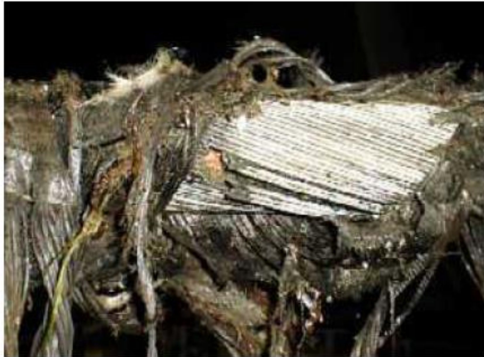
Anchor damage on Baltic Cable
