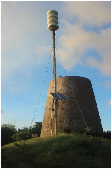
*Picture 4: Volcanic Activity Monitor Siren Powered by Photovoltaics on the outskirts of Plymouth and the No Entry Zone*
